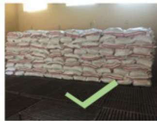
Stacking of HDPE bags by Brick layer method
